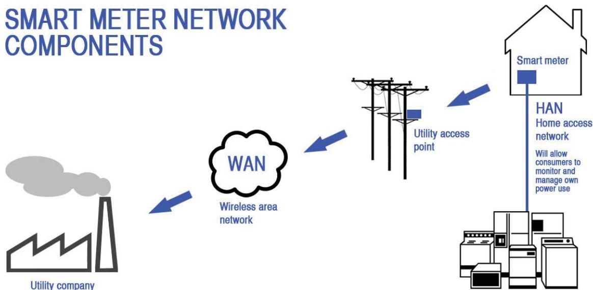
**Figure 3. Simplified depiction of Smart Meter system network. Arrows show the use of radiofrequency (RF) signals for automated meter reading, communications among electric power meters, relays, access points, the company’s enterprise management systems. The future home access network will operate within the house.**
