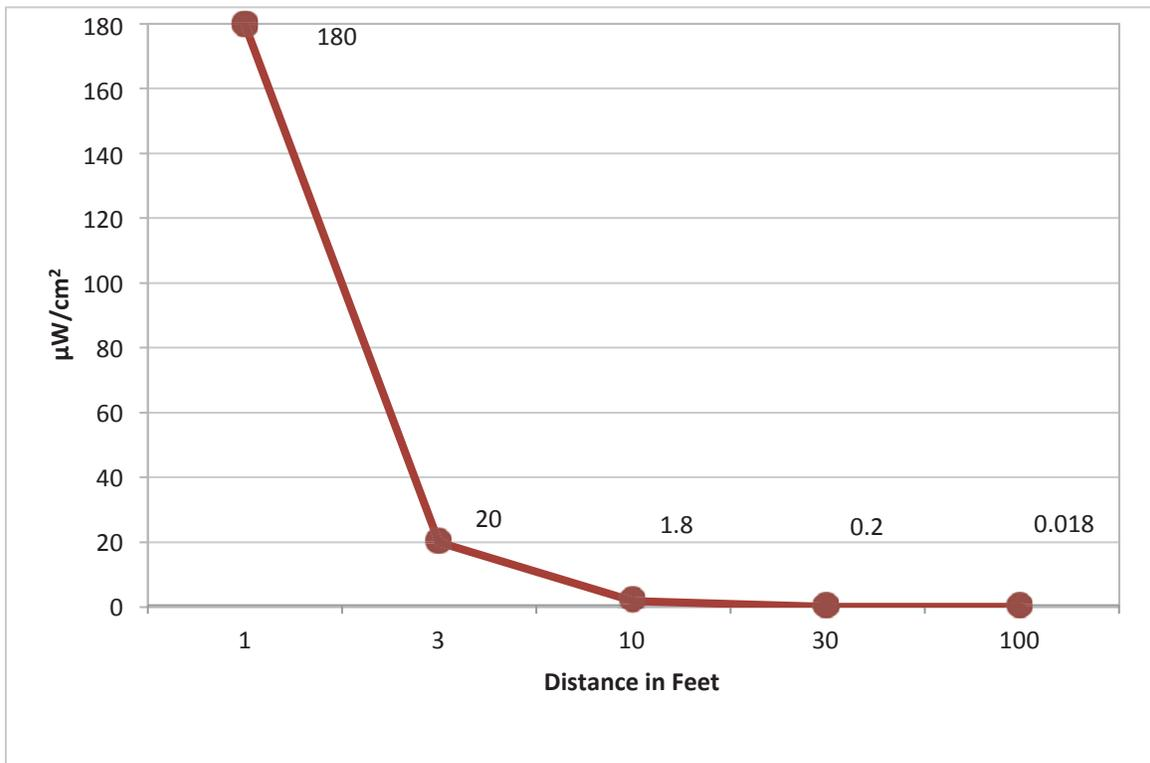
**Figure 6. Power density from a sample smart meter versus distance;<sup>30</sup> 1-Watt emitter at 50% duty cycle. Typical smart meter AMR transmitter power density declines rapidly with distance. The rapid drop of power density with distance (inverse-square law) is similar for various duty cycles and different sets of source data.**
