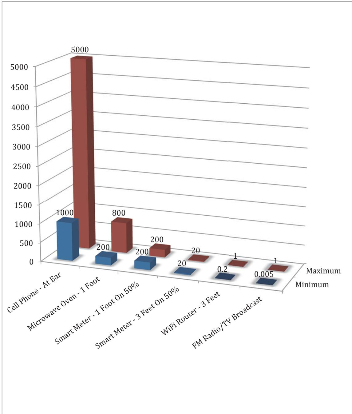
**Figure 1. Instantaneous Radio Frequency Power Density Levels of Common Devices (in microWatts/cm<sup>2</sup>)**
