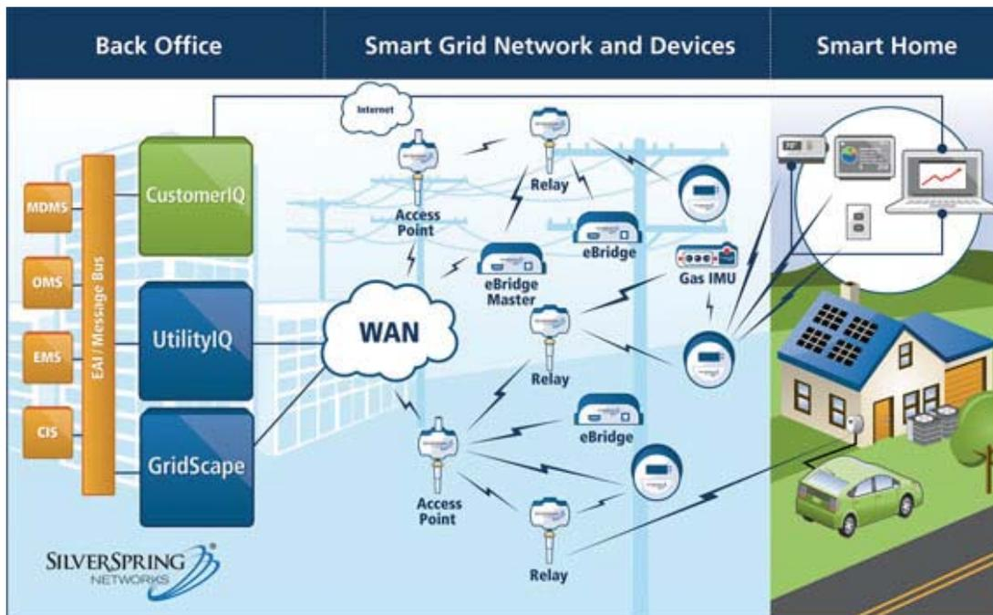
**Figure 4. Illustration of components of the PG&E Smart Meter Program Upgrade showing the use of radiofrequency (RF) signals for communications among electric power meters, relays, access points and, ultimately, the company’s enterprise management systems. (Source Silver Spring Network<sup>5</sup>)**
