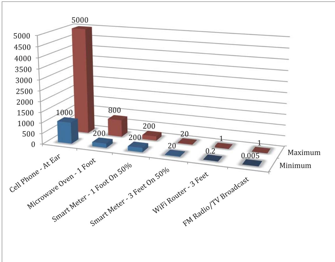
**Figure 7. Instantaneous Radio Frequency Power Density Levels of Common Devices (in microWatts/cm<sup>2</sup>)**
