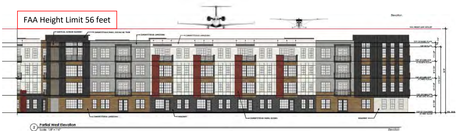
Figure 2 Proposed Elevation diagram for Modern West Development. Note the red line above the building. That is the bottom of the protected area by the FAA for aircraft (40:1) at 56 feet. Someone on the roof might have to duck when aircraft fly over. A Cessna 172 (typical aircraft at KLMO) and an Embraer Phenom 300 aircraft are overlaid for scale (largest based aircraft at KLMO) at the height that they could in principle cross over the development for landing and meet the FAA requirements.
